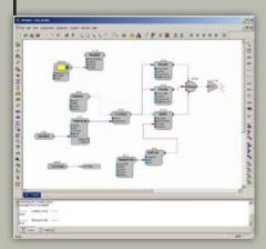
can be loaded and controlled from TDT software applications. By allowing run-time access to these processing chains, RPvds gives you a level of real-time control not available in other systems.
