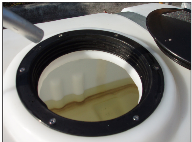
Figure 7.4: Tanks should have a large opening for ease in filling. Credit: UF/IFAS Pesticide Information Office.
