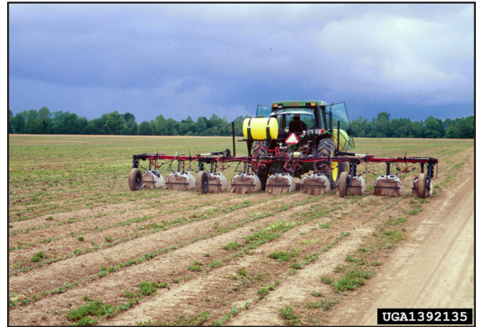
Figure 7.13: Sprayer with shields. Credit: Charles T. Bryson, USDA Agricultural Research Service, Bugwood.org.
