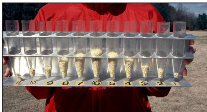
Figure 8.9: Typical pattern seen from a double-spinner spreader. Credit: Wayne Buhler, N.C. State University.
