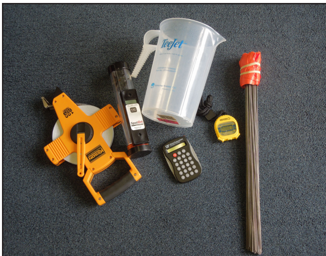
Figure 8.2: Some of the simple tools needed for calibration. Credit: UF/IFAS Pesticide Information Office.
