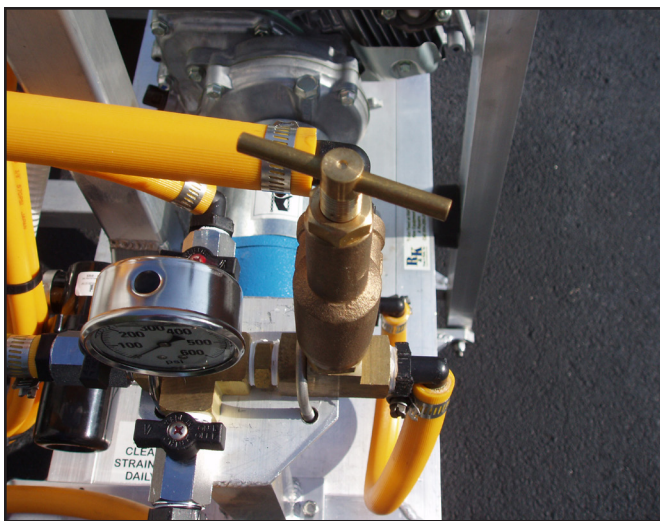
Figure 7.9: Spring-loaded pressure relief valve. Credit: UF/IFAS Pesticide Information Office.
