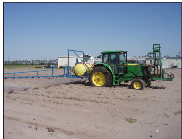
Figure 7.1: Large low-pressure sprayers are commonly used in row crop agriculture. Credit: UF/IFAS Pesticide Information Office.
