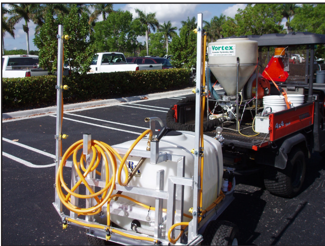
Figure 7.3: Boom sprayer equipped with a hand spray gun attachment. Credit: UF/IFAS Pesticide Information Office.
