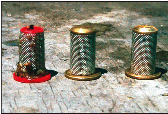
Figure 7.7: Left to right: strainer with debris; strainer with leftover pesticide, and clean strainer. Credit: UF/IFAS Pesticide Information Office.
