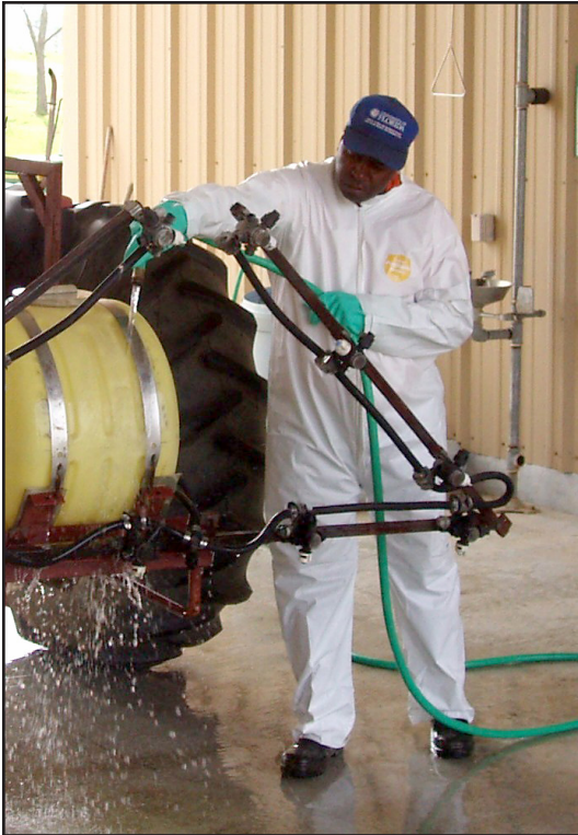
Figure 5.18: Washing a spray rig on a concrete containment pad. Credit: UF/IFAS Pesticide Information Office.
