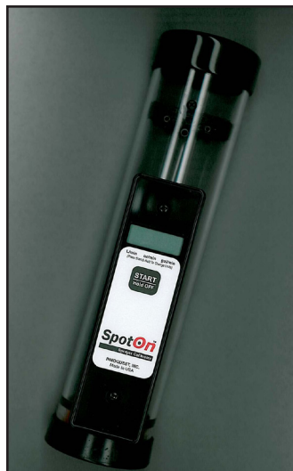
Figure 8.5: Handheld device for checking nozzle output. Credit: UF/IFAS Pesticide Information Office.
