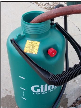
Figure 5.15: Never do this; always leave an air gap—it's the law! Credit: UF/IFAS Pesticide Information Office.
