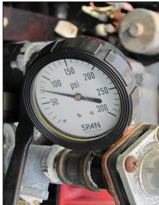
Figure 7.10: Pressure gauge with a 300 psi maximum reading capacity. Credit: UF/IFAS Pesticide Information Office.
