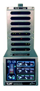
Overview. The PZ5 is a multi-modal neurodigitizer suitable for recording a broad range of biological potentials. analog input boards combine the functionality of the PZ2 and PZ3 amplifiers in a single device that can be used for both high and low impedance input signals simultaneously. The PZ5 may also include digital input boards for inputting signals from an Intan RHD2000 amplifier board with up to 128 channels.
